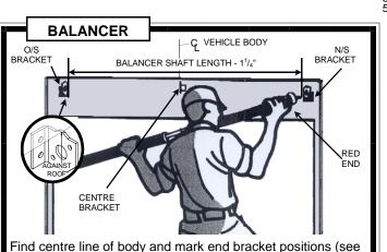
diagram.) Weld or bolt brackets as close to roof as possible. Insert balancer with red end on the right (viewed from inside the body.) Insert split pins on either side of right hand bracket and open out to retain in position.
