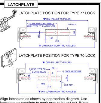
latchplate as template to mark area to be cut out. When fitted, the upper face of the latch plate MUST be flush with and parallel to the surface the door closes against. The latch plate can be welded or bolted in place.
