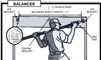
Find centre line of body and mark bracket positions (see diagram.) Weld or bolt brackets as close to roof as possible. and open out to retain in position.
