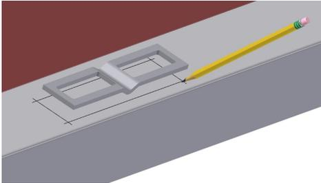
Cut sill if necessary. Position evenly flush with top surface of sill (**very important**).
