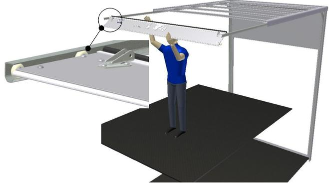
This section can be rolled along the complete track assembly keeping it perpendicular to check the track spacing throughout.
