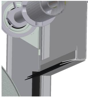
Top seal, fitted to underside of header
