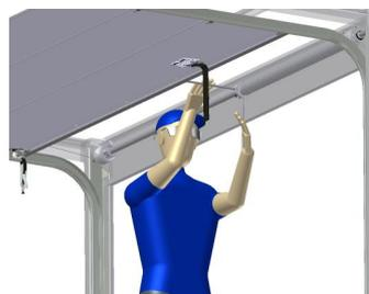
Using the holes in spring torque casting & two tommy bars in a upwards direction add 6 turns.
