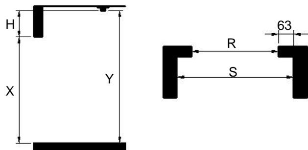
**Dimension X: Sill to header**, vertical distance between underside of header and sill (surface on which door is resting when closed)
