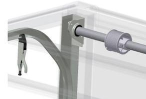
Place a single spacer washer and rollers in an inter panel, check inter seal is in place and engage the joint, rotate up and position rollers in the end of the track by pushing assembly further along the horizontal track.
