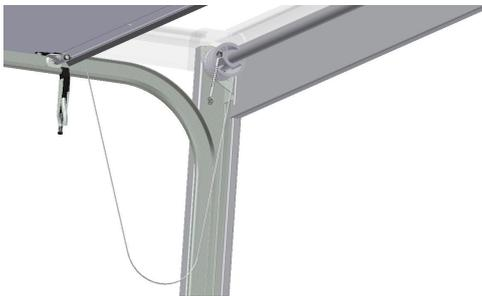
Slacken off cable drum set screws.
