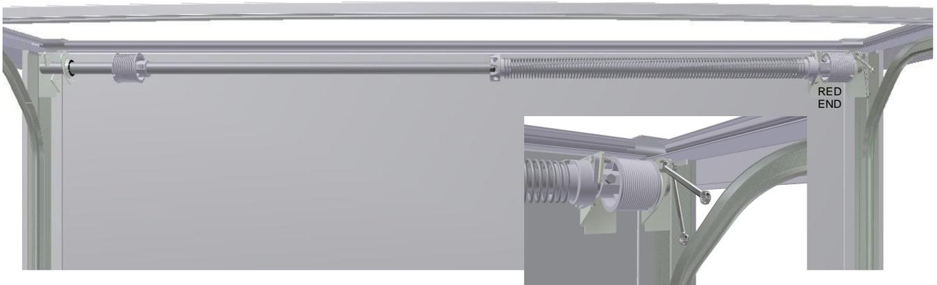
Fully Secure **all** bearing fixings and torque to 6N/m.
