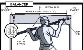
Find centre line of body and mark end bracket positions (see diagram.) Weld or bolt brackets as close to roof as possible. Insert balancer with red end on the right (viewed from inside the body.) Insert split pins on either side of right hand bracket and open out to retain in position.
