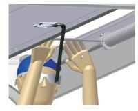
Slacken the two square head bolts in spring torque casting.
