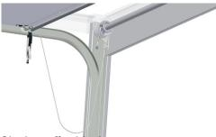
Slacken off cable drum set screws.
