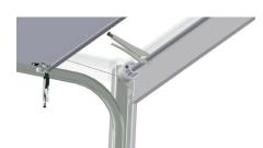
Before winding cable onto other drum. Place a pair of mole grips onto balancer shaft to prevent cable from unwinding.
