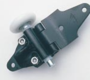
End hinge assembly c/w removable roller clamp to allow roller change in situ
